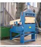
The Classifier is perfect for recovery of metals remaining in the plastic fraction. Reduction of metal losses down to 2.0%
