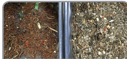
Copper Wire from ECS Fines
